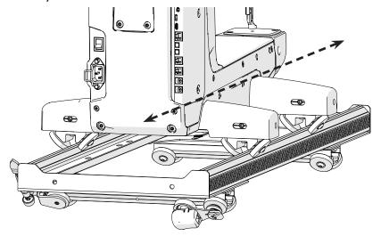
11 Use the 4 mm Allen wrench to re-tighten the wheel assembly set screws you loosened earlier.
