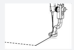
b Hold the thread to make a loop and return the machine to the tie-off stitch.
