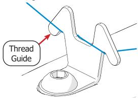
3 Pull the thread through the hole in the **tensioner thread guide** and then around the back of the **bobbin thread tensioner**, between the two discs.
