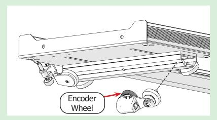
d Turn the encoder **lock collar** (shown in blue) to point up. Then tighten the **lock collar screw** with the 2.5 mm Allen wrench.
