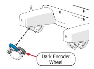
6 Tighten the **encoder screw** with the 4 mm Allen wrench.
