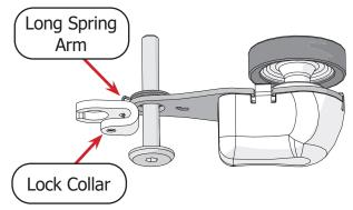
7 Place the replacement spring over the encoder screw, and insert the **short arm** of the spring all the way through the hole on the encoder base.
