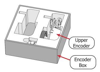
3 Loosen the **lock collar screw** on the upper encoder with the 2.5 mm Allen wrench until the **lock collar** (shown in blue) turns freely.
