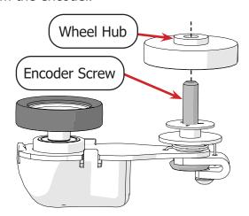
5 Place the encoder screw into the left rear wheel hole so the **dark encoder wheel** is between the two left machine wheels.
