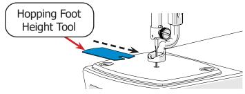
**Note:** The height tool prepares the machine for standard sized quilt batting and two layers of fabric. For thicker quilts, stack sheets of printing paper over the gauge to increase room underneath the hopping foot.
