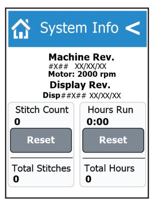
**Tip:** It's recommended to oil your machine after 20 hours of use. The "Hours Run" counter can help keep track of when your machine is due to be oiled. After cleaning and oiling your machine, press the **Reset** buttons under "Hours Run" and "Stitch Count" to start the counters back at zero.
