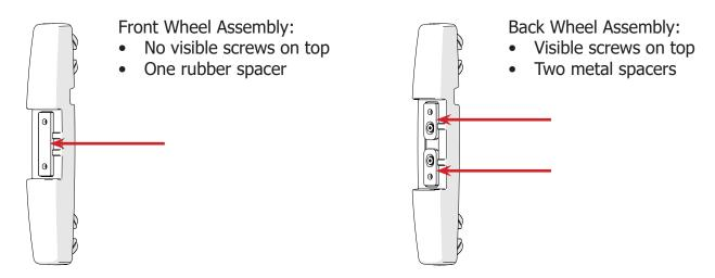
6 Attach the front wheel assembly to the bottom of the machine with the two **M6 shoulder bolts** and the 4 mm Allen wrench. Make sure the **holes** in the back of the wheel assembly are facing towards the back.
