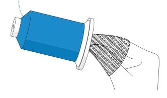
5 Use your fingers to widen the lower part of the thread net and wrap it around the base of the thread cone. The thread net should cover at least the bottom half of the thread cone.
