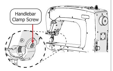
The handlebar clamp opens.
