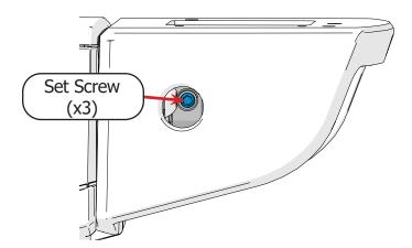
6 The **outside** part of the hook assembly (shown in blue) now rotates by hand. Turn the outside part of the hook assembly so that the **hook** is at the top.
