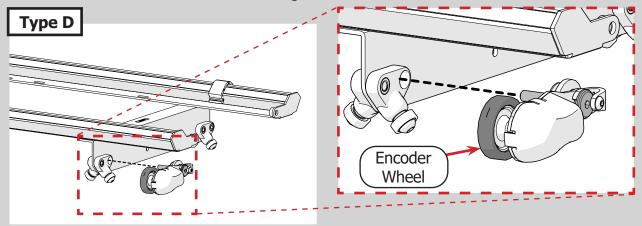
© Turn the encoder **lock collar** (shown in blue) to point up. Then tighten the **lock collar screw** with the 2.5 mm Allen wrench.
