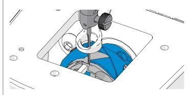
9 Slip the timing spacer tool (shown in blue) into the hook assembly with the flat side facing up. Then turn the timing tool until the flat side faces down.
