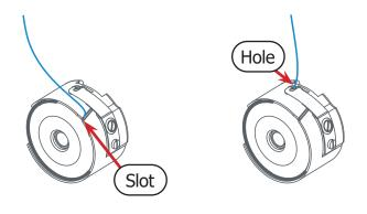
**Note:** If the bobbin is wound correctly it will turn clockwise when the thread is pulled.
