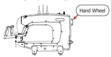
2 Slide the **needle plate** (shown in gray) onto the machine.
