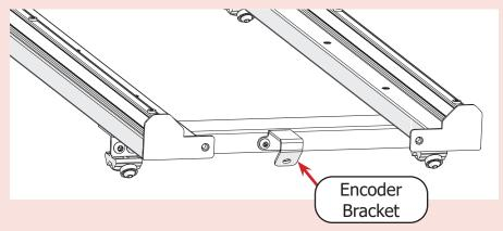
(b) Install the encoder directly onto the encoder bracket at the rear of the carriage so the **encoder wheel** is to the left of the bracket. Tighten with the 4 mm Allen wrench.
