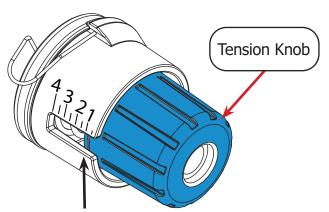
**Note:** Setting "1" is the lowest tension for your machine, and is an ideal starting place to find the correct top tension.
