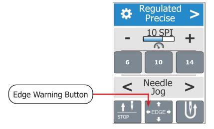
**Note**: Edge Warning is automatically deactivated in Baste Mode.
