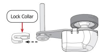
8 Place the **long arm** of the encoder spring arm into the hole on the encoder **lock collar**.
