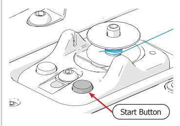
5 Winding stops automatically when the bobbin is full. Cut the bobbin away from the thread cone using the **thread cutter** near the bobbin winder.
