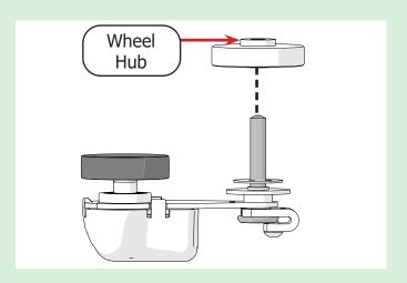
c With the 4 mm Allen wrench, screw the encoder into the left rear wheel hole on the carriage so the **encoder wheel** is between the rear wheels.
