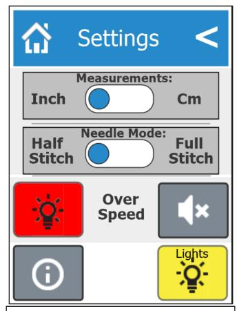
**Note**: The machine is unable to stitch while the Tools or Settings menu is pulled up.
