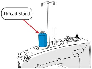
4 Pull the thread straight up, through the **thread mast guide loop** above the thread stand.
