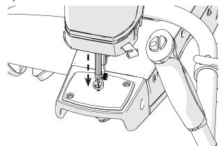
4 Align the screw holes on the needle plate with those on the machine.
