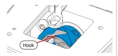
7 Carefully rotate the hand wheel to drop the **needle** (shown in gray) all the way to the lowest point. Continue rotating the hand wheel the same direction. The **needle** should begin to raise up.
