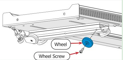
(b) Install the wheel onto the encoder bolt so the **wheel hub** is away from the encoder.
