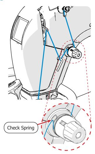
8 Next, pass the thread down and around the **thread guide** next to the large thread tensioner.
