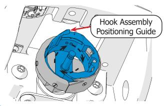
5 Slide the **finger** of the **hook holder** into the middle of the **hook assembly's positioning guide** (shown in blue).
