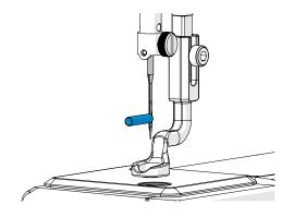
7 Hand-tighten the **needle thumb screw**. Do not over-tighten if using the flat-head screwdriver.
