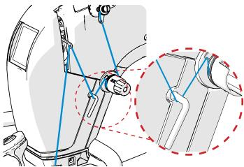
9 Pull the thread through the hole in the takeup lever.
