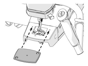
3 Slowly lower the needle with the hand wheel. The needle should slide into the center hole without contacting the needle plate.
