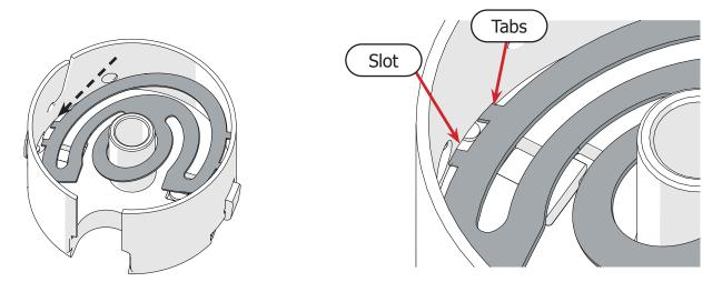
4 Press the other side of the spring down and insert the other tabs on the other side. Use the small flat-head screwdriver to make sure all four tabs are fully secured.
