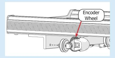
d Turn the encoder **lock collar** (shown in blue) to point up. Then tighten the **lock collar screw** with the 2.5 mm Allen wrench.
