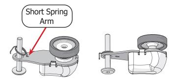
9 Without allowing the arm to slip out of the lock collar, rotate the collar until it wraps around the encoder bolt.
