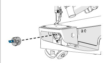
4 Look into the machine's **timing cut-out** and turn the hand wheel. The **hook assembly** will rotate.
