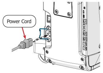
3 Press the **power cable retainer** (blue) firmly onto the power cable.
