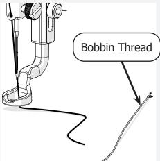
e Pull on the bobbin thread while moving the machine back to the start point. This makes sure that there is no loose thread underneath the fabric.
