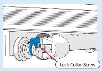
e Take the free end of the **encoder cable** (shown in blue) and pull it through the slot in the bottom carriage behind the wheels.
