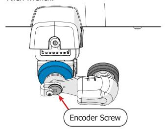
7 Turn the **encoder lock collar** (shown in blue) to point up and tighten the **lock collar screw** with the 2.5 mm Allen wrench.
