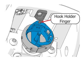
6 Attach loosely with the **hook holder screw**. Do not tighten.
