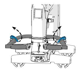
7 Twist the controls vertically until they are comfortable to hold and operate.
