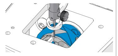
8 Stop raising the needle once the eye is about level with the **hook** (shown in blue). Do not continue to raise the needle. If the needle reaches the top of its rotation (over the hopping foot), start over at step 7.
