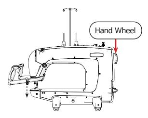
2 Use the 3 mm Allen wrench to loosen, but not remove, the **hopping foot screw**.
