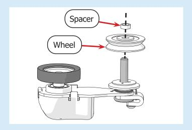
with the 4 mm Allen wrench, screw the encoder into the left rear wheel hole on the carriage so the **encoder wheel** is between the rear wheels.
