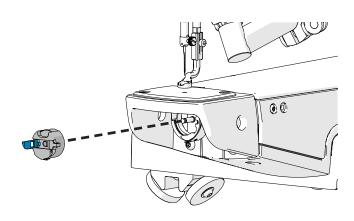
4 Turn the inside part of the **hook assembly** (shown in blue) so that the **positioning guide** is at the highest point.
