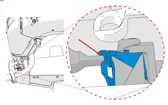
8 Tighten the hook holder screw to fasten the hook holder in place. The inside part of the hook assembly should no longer rotate freely by hand.
