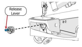
5 Set the bobbin aside. Clean the bobbin case with the lint brush or compressed air. Be sure to clean the area under the **bobbin tension thread arm**.
