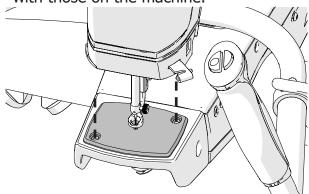
5 Place the two **needle plate screws** (shown in gray) into the plate. Make sure the needle plate is centered around the needle, and then tighten the screws with the flat-head screwdriver.
