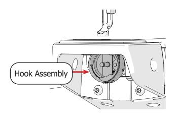
7 Rotate the **hand wheel** until the needle is halfway down. This will put the hook in the best position for oiling.
