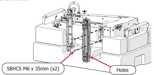
8 Remove the machine from the packaging and place it on the bottom carriage on the frame.
