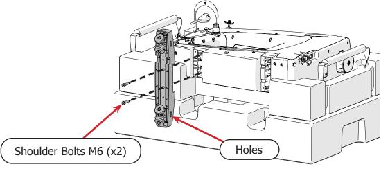
Attach the back wheel assembly to the bottom of the machine with the two **M6 x 35 SBHCS** and the 4 mm Allen wrench. Make sure the **holes** in the back of the wheel assembly are facing towards the back.
