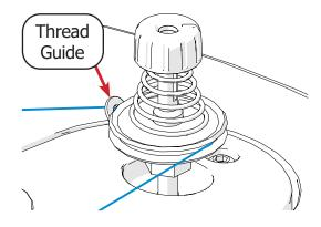
4 Wrap the thread clockwise around the empty bobbin. Press **start** when ready.
