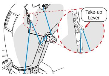
10 Then pass the thread down through the **bottom thread guide** on the way to the needle.
