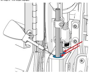
11 Power up the machine and run it for about ten seconds to evenly spread the oil around the hook assembly.
