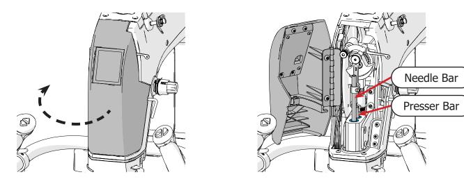
10 Place 1-2 drops of oil at the bottom of the needle bar and presser bar where they meet the bushing block.
