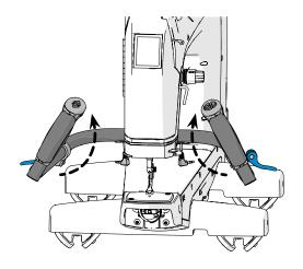
8 If desired, extend the handles outward to improve the reach of the machine.
