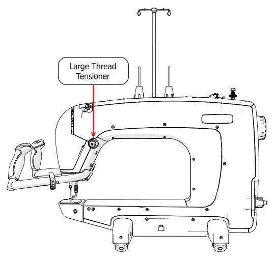
1 Loosen the **tension knob** on the **large thread tensioner** to set the tension to "1." The bottom of the tension knob will line up with the number that the tension is set to.
