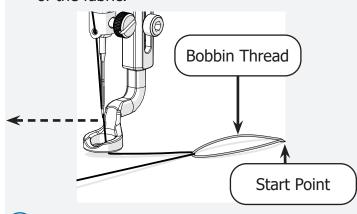
d Pull on the loop of **bobbin thread** until the loose end of the thread comes up from underneath the fabric.
