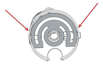
5 Place the **bobbin** in the bobbin case. The anti-backlash spring should hold the bobbin so that it barely pokes out of the opening of the bobbin case.
