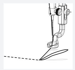
e Keep moving away from the tie-off until a loop of bobbin thread is pulled up above the fabric. Cut all threads close to the tie-off.
