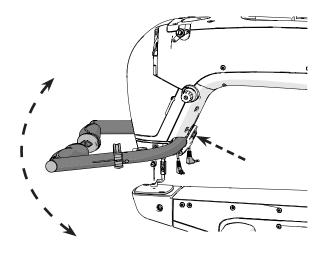
6 Open the **handlebar levers** (shown in blue).
