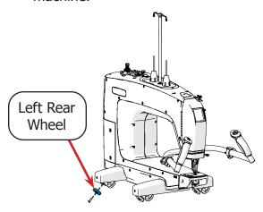
The **wheel screw** will not be needed again and can be stored with the packaging materials.
