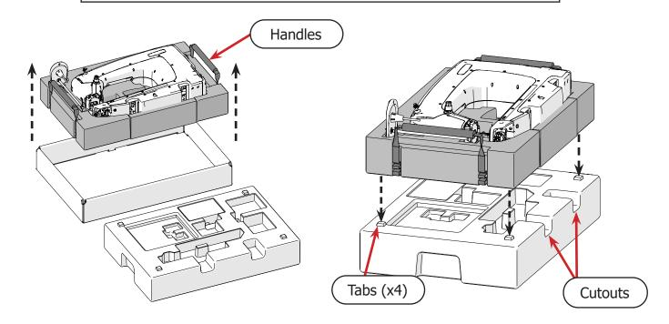
4 Remove the piece of **foam** covering the bottom of the machine.
