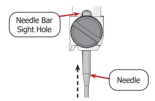
5 The **scarf**, a cut-out on the back of the needle, should face the throat of the machine. Place the **needle magnet** on the opposite side of the scarf.
