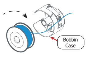
5 Slip a few inches of thread through the **slot** and out of the **hole**.
