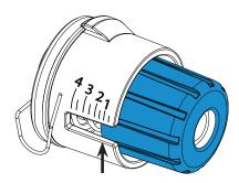
• If the **top thread** is pulled down through the bottom layer of fabric, there is too little top tension. Increase the tension on the top by slowly turning the large thread tensioner knob toward setting "4." Stop turning the knob when desired tension is achieved.
