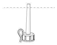
2 Place the applicator needle onto the top of the cap.
