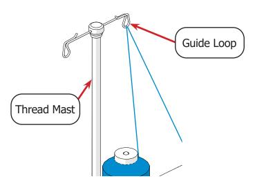
2 Pass the thread underneath the left side of the **thread guide**. Move it through the middle of the thread guide back to the front and then underneath the right side of the thread guide.
