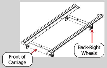
b Use the 5 mm Allen Wrench to remove the **wheel screw** and the **M6 spacer** from the back of the back-right **wheel holder**.
