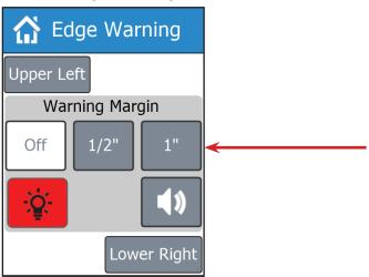
5 The arrows on the edge warning button in the quilting mode screen will turn green when edge warning is activated.
