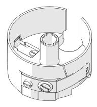
2 Position the **anti-backlash spring** so that the **center** section is raised above the edge of the spring.
