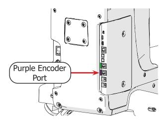
9 Plug the lower encoder cable into the green encoder port on the left rear of the machine.
