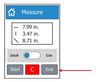
6 Press the **clear** button once you no longer need to save the measurement or if you are ready to make a measurement with a new start point.
