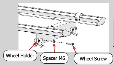
**Note:** The **wheel screw** is not needed again and can be stored with the packaging materials.
