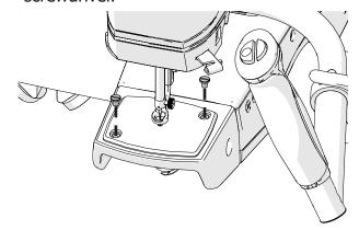
6 Use the **hopping foot height tool** to adjust the height of the hopping foot.
