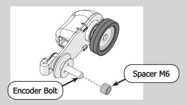
Install the encoder directly onto the wheel holder at the rear of the carriage so the **encoder wheel** is to the left of the bracket. Tighten with the 4 mm Allen wrench.
