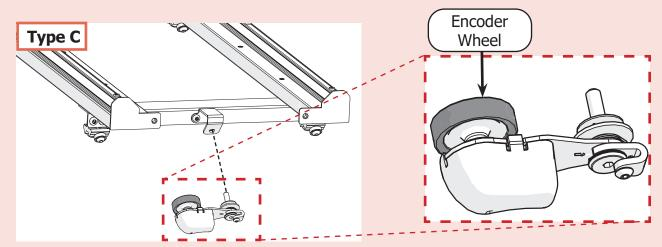
Turn the encoder **lock collar** (shown in blue) to point up. Then tighten the **lock collar screw** with the 2.5 mm Allen wrench.
