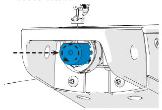
Turn the hand wheel the opposite direction to bring the **needle** back down until it rests on top of the **timing spacer**. Do not let the **needle** rise to the top before bringing it back down or you will need to repeat steps 7-10.
