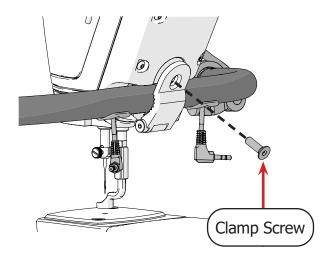
5 Hold the handlebars at the desired angle and tighten the clamp screw.
