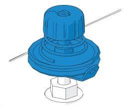
4 Once the bobbin is filling correctly, re-tighten the **nut**. Make sure the **thread guide** is on the correct side of the tensioner assembly.
