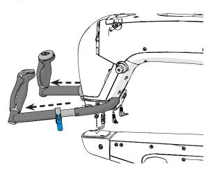
Once you are comfortable with the position of the handles, close the **handlebar levers** (shown in blue).
