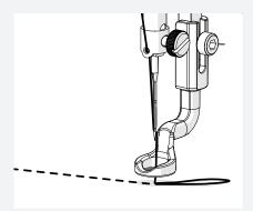
d Hold the loop and move the machine away from the tie-off again.
