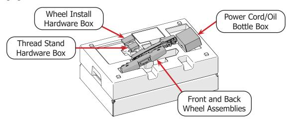
2 Lift the top layer of packaging and place it beside the bottom layer that holds the machine.
