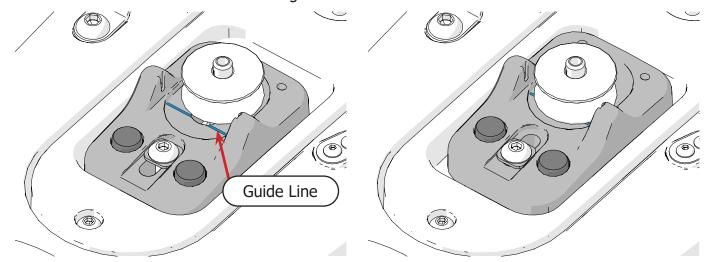
$\bigcirc$  Tighten the M5 x 16 mm SBHCS to secure the bobbin winder in place.
