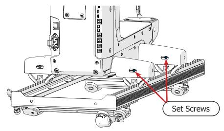
10 Roll the machine up and down the bottom carriage tracks several times so that the machine can settle and ride smoothly.
