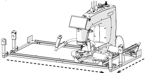
**Cutie frame users only:** Use a **zip tie** to fasten the power cord to the back left **hole** on the Cutie frame carriage. The power cord should have a little bit of slack between the zip tie and the machine.
