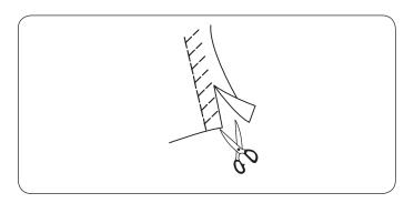
Place your fabric to allow a  $5/8^{\circ}$  (1.5 cm) seam. Trim excess close to the stitching. Be careful not to cut the stitches.
