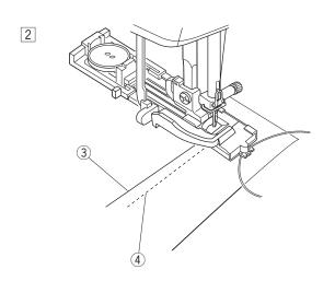
2 Start the machine and sew the buttonhole.
