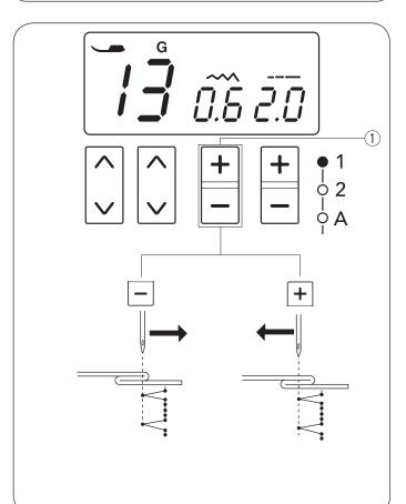
Adjust the needle drop position as follows:
