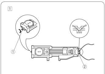
1 Use the same procedure as the square buttonhole sewing. Set the stitch width to match the thickness of the cord used.
