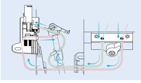
when the lever reaches the bottom. This ratchet type air thread system creates optimal conditions for achieving reliable air-threading.
